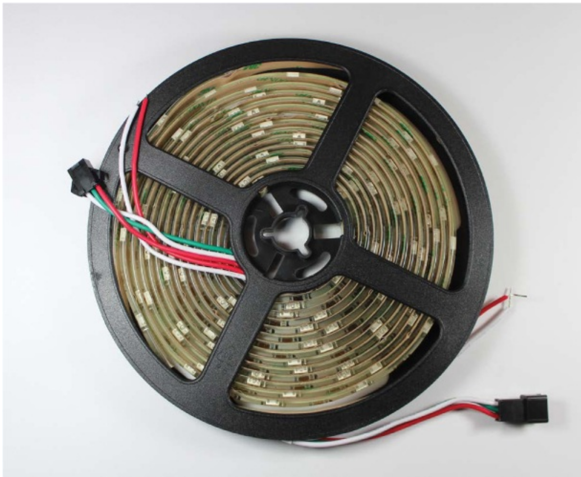
FIGURE 5-1: WS2812B addressable RGB LED strip on a reel The strip shown in Figure 5-1 is 5 meters long with 300 addressable WS2812B RGB LEDs wired in series, and later you'll cut a section of 14 LEDs to use in this project. There are cutting marks, shown in Figure 5-2, along the entire length of the strip.
