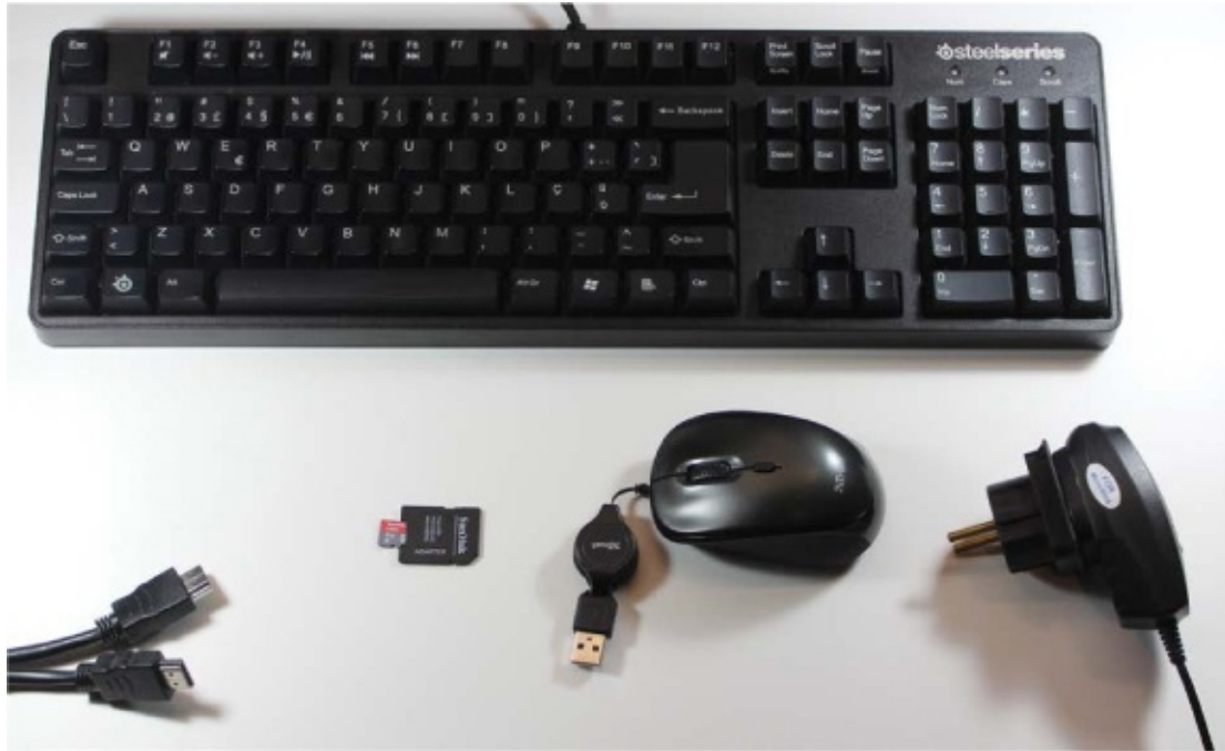
FIGURE 0-5: A keyboard and, from left to right, an HDMI cable, a microSD card, a mouse, and a power adapter Here's a list of things you'll want to purchase for the Pi: Power adapter
