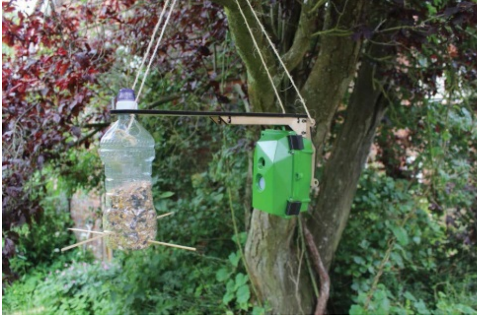
FIGURE 13-2: Raspberry Pi camera with PIR motion sensor pointed at a bird feeder
