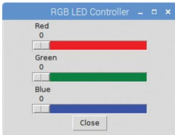
FIGURE 4-5: The RGB LED controller user interface Congratulations! You've made your own component user interface! Now try moving the sliders to change the LED color. When you change each slider's position, the RGB LED color should change accordingly.
