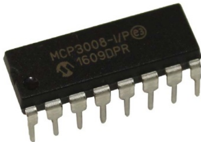
FIGURE 3-3: MCP3008 chip analog-to-digital converter This chip has 16 pins, 8 of which are analog inputs you can connect to analog devices. The other 8 connect to the Raspberry Pi GPIOs. The chip pinout is shown in Figure 3-4. To identify each pin, orient the chip with the half-circle at the top as shown in the figure.
