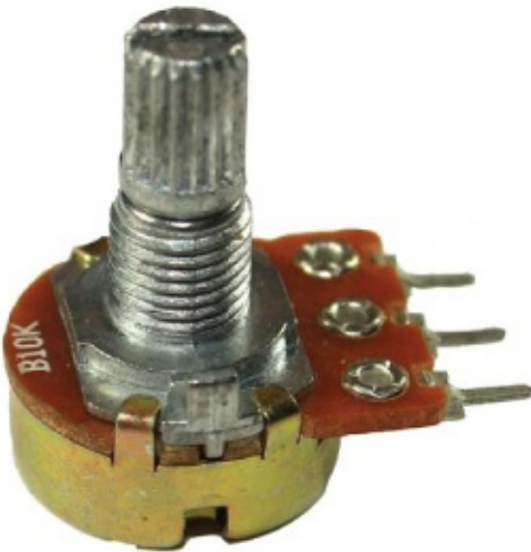
FIGURE 3-1: A 10 k \Omega potentiometer A potentiometer, also referred to as pot , is a manually adjustable variable resistor. This means that you can change the amount of resistance it applies to a circuit by rotating the knob, changing the amount of current reaching a particular component.
